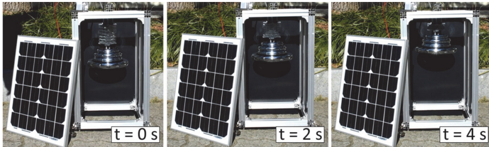
Figure 2-14. The actuator with a payload of 10 kg driven using a 17.7 V solar panel.
