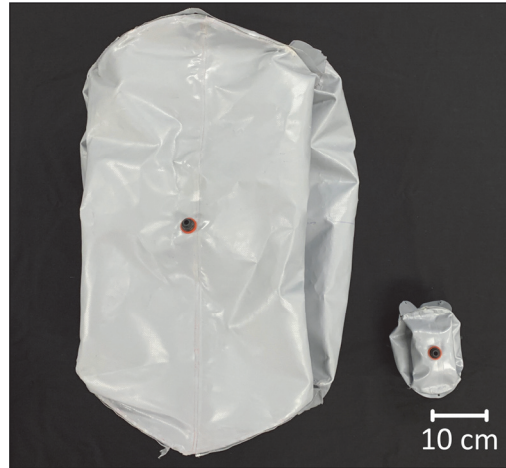
Figure 3-43. Inflatable joint element with a diameter of 40 cm and a height of 40 cm.
